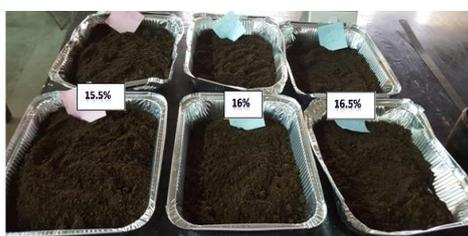
**Figure 3.** Aeration of asphalt stabilized mixture
