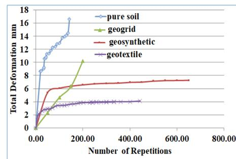
Figure9. Total deformation under wheel tracking test
