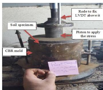
Figure6. Test setup
