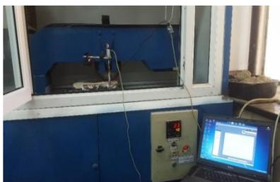
Figure7. Wheel tracking apparatus
