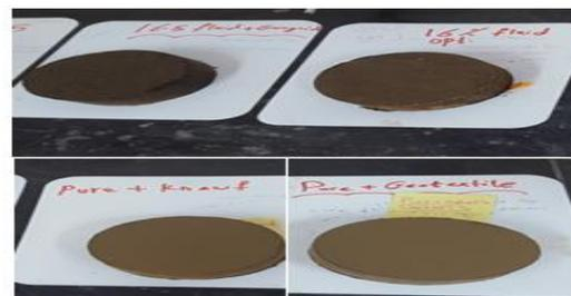
**Figure 4.** Part of Specimens of wheel tracking test under curing
