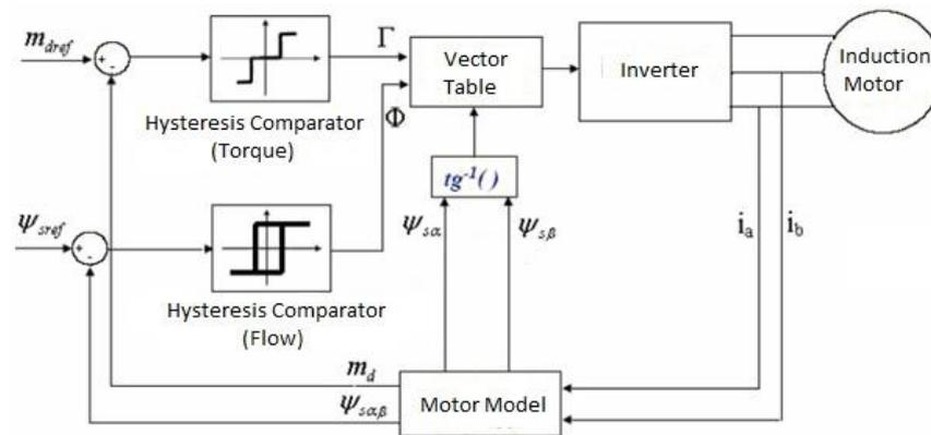
Figure6. Structure of direct torque control system
