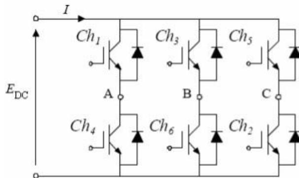
**Figure4.** Scheme of voltage source inverter
