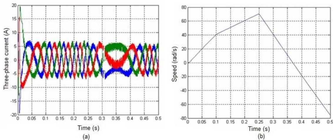
Figure10. (a) Simulation results of three-phase stator currents, and (b) Motor Speed by the proposed DTC algorithm
