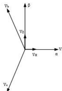
**Figure3.** Inverse Clarke transformation from two phases to three phases
