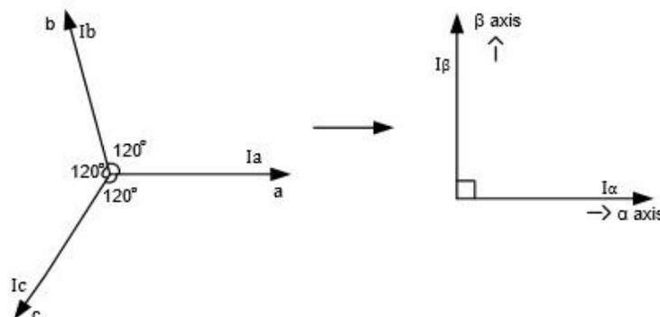
Figure2. Clarke transformation from three phases to two phases
