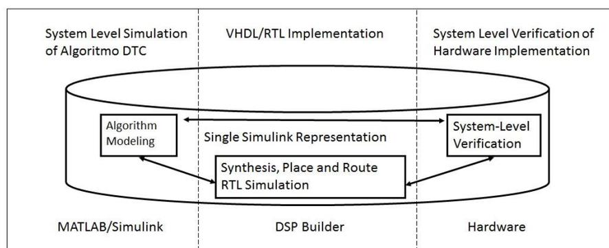
Figure7. Design flow with the MATLAB/Simulink and DSP Builder
