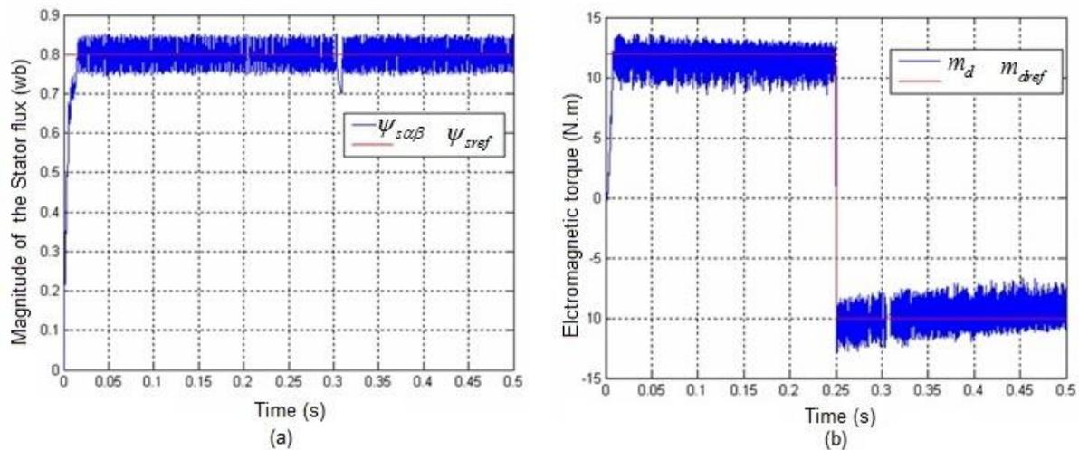
Figure9. (a) Simulation results of stator flow estimated, and (b) Electromagnetic torque estimated by the proposed DTC algorithm
