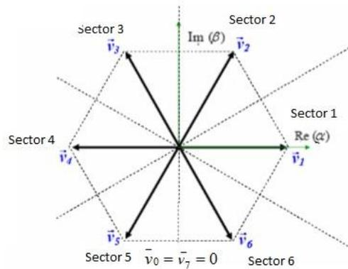
Figure 5. Voltage space vectors generated by the VSI
