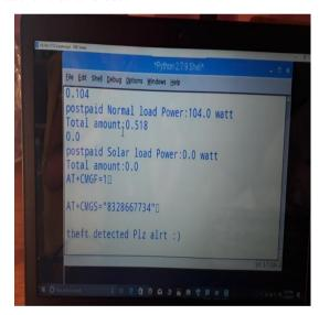
Fig2. Alert with SMS both user and service provider
