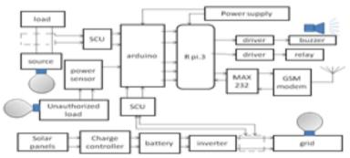
Fig1. Block diagram for bidirectional meter
