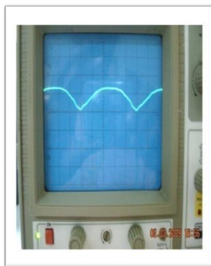
Fig 8.1. Bridge rectifier output
