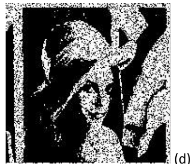
Fig1. A 2-out-of-2 VCS using additional pixel patterns (a) the original image, (b) the first share S_1 , (c) the second share S_2 , and (d) superimposed S_1 and S_2 .
