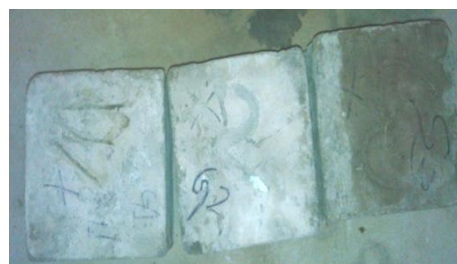
Fig 5. 20% of glass replaced to sand
