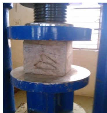
Fig 6. Compressive test on concrete
