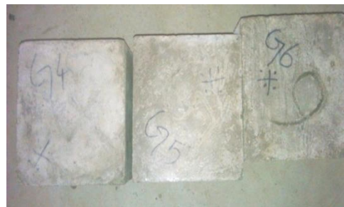
Fig 4.. 15% of glass replaced to sand
