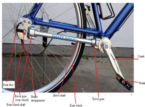
Fig3.1. components of shaft driven bicycle
