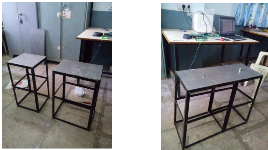
Fig 2. Three Framed Structure and Structure Connected with FFT Analyser
