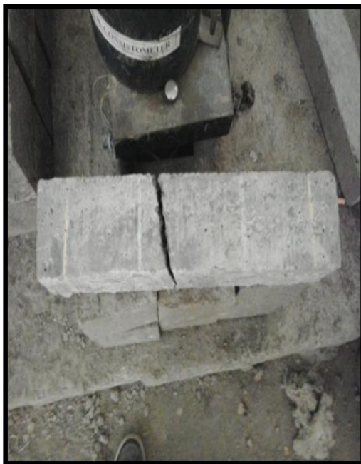
Figure 6. Failure of Plain Cement Concrete Beam (28 days)
