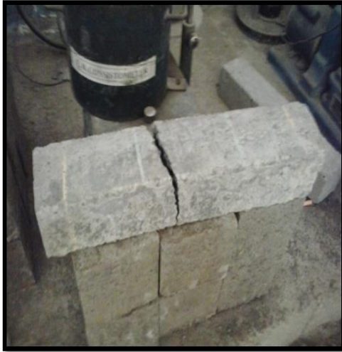
Figure 2. Failure of Plain Concrete Beam.(7 days)
