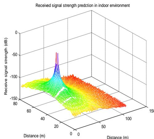
**Figure 6.** Distance vs. Received Signal Strength at  $F = 1.8 \text{ GHz}$ .
