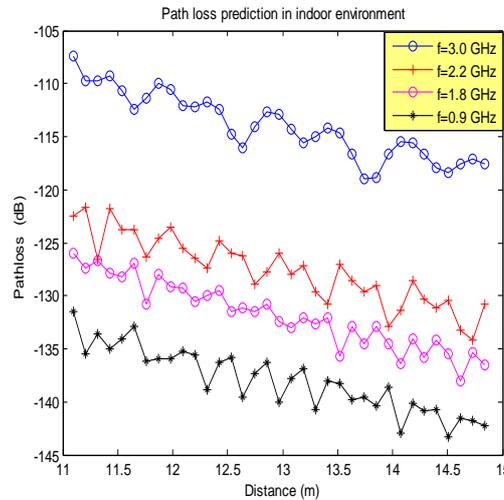
**Figure 4.** Distance Vs Path loss at different frequency for indoor scenario in figure (3).
