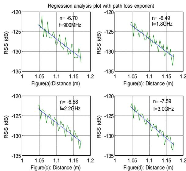
**Figure 5.** Distance vs. Received Signal Strength (RSS) Regression Curve at 900 MHz, 1.8 GHz, 2.2 GHz And 3.0 GHz
