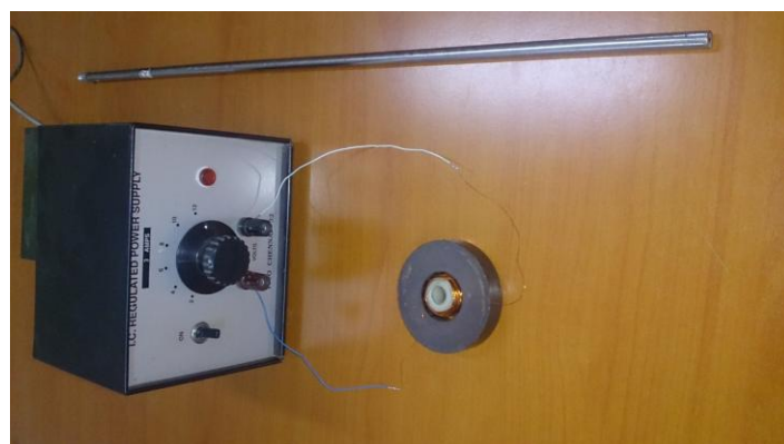
Fig.3. Photograph of coil housed inside the centre hole of circular magnet.
