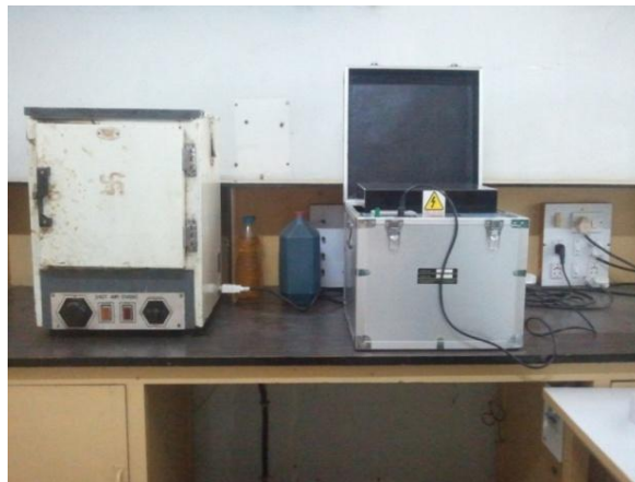
Figure 2. Experimental setup with Automatic transformer oil testing kit
