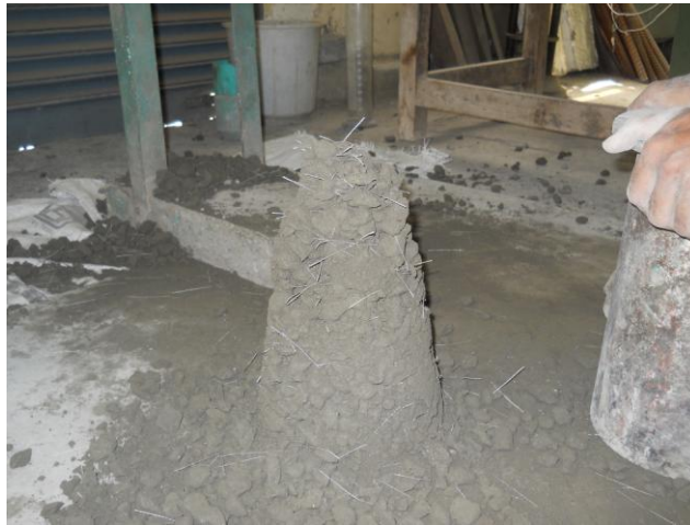
Shear failure during slump test
