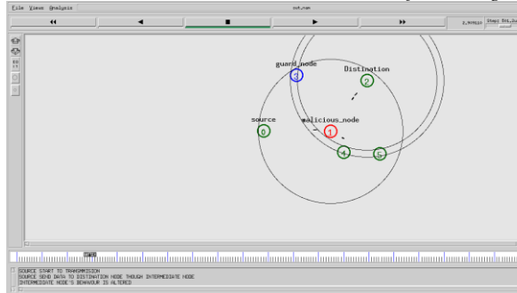
Fig.15 .Node 5 also sends a packet to intermediate node, due to this collision will occur
