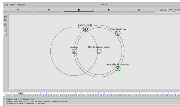
Fig.6. Intermediate node become malicious node due to misrouting attack
