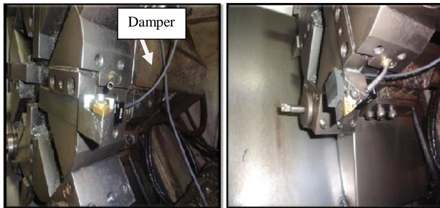
Diagram shows tool without and with damper
