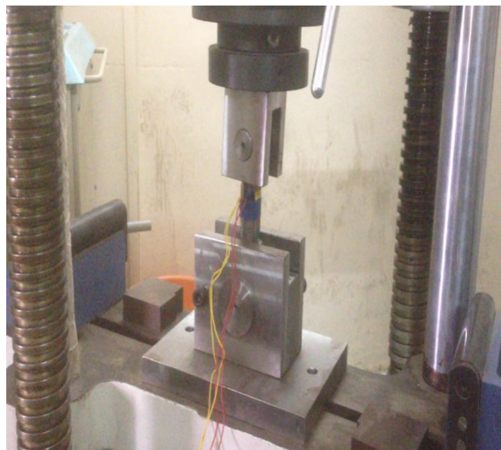
Fig2. Arrangement of fixture for holding connecting rod
