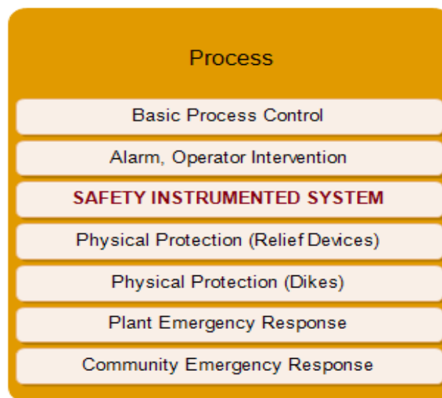
Figure 2. Safety Protection Layers.
