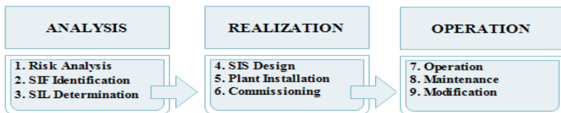
Figure 1. Simplified Block Diagram of Safety Life Cycle
