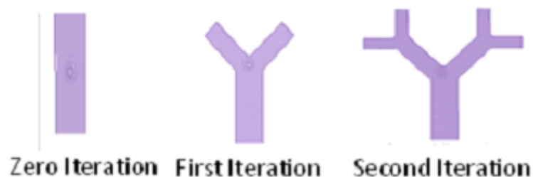
Fig3. Process of making fractal tree antenna
