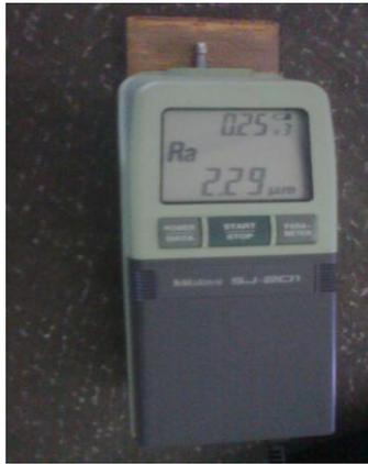
**Figure 4.** Portable Surface Roughness Tester
