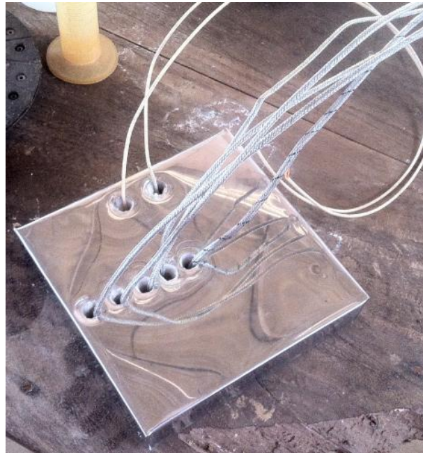
Figure 4. Five thermocouples radially connected
