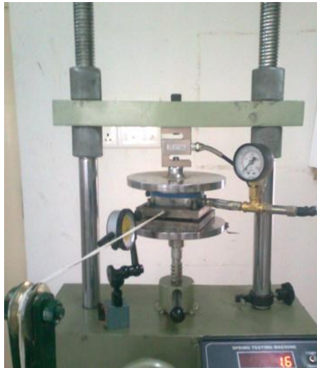
Figure 5. Slip and shift testing set up for robot fingers
