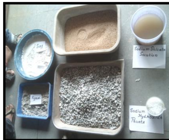
Figure 1. Materials used for preparing Geo-polymer concrete
