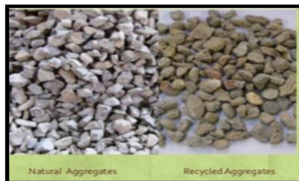
Figure 2. Natural aggregate and Recycled aggregate
