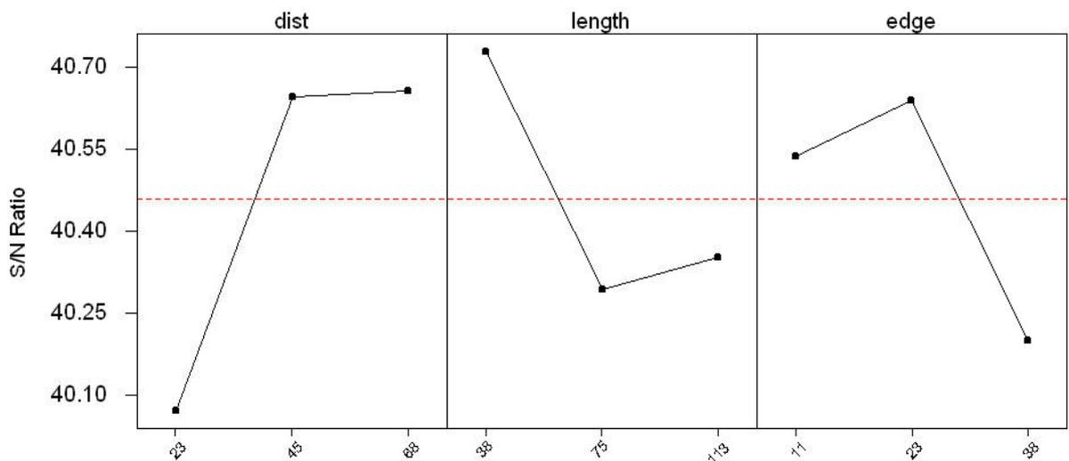
Fig3.2.2. Main effect plot for means for average tensile strength
