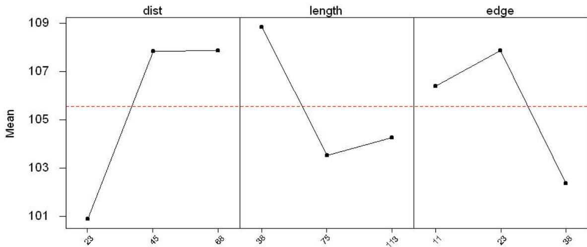
Fig3.2.1. Main effect plot for means for average tensile strength
