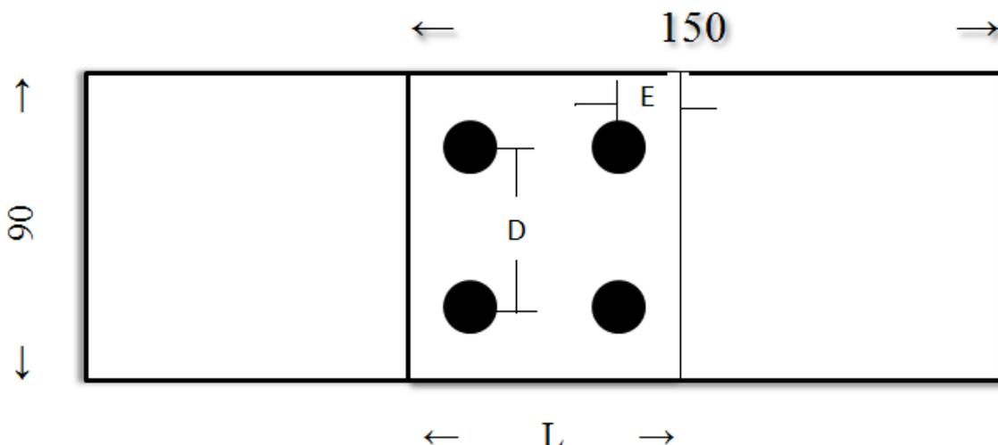
Fig2.1. Dimensions of Specimen (all dimensions in mm)
