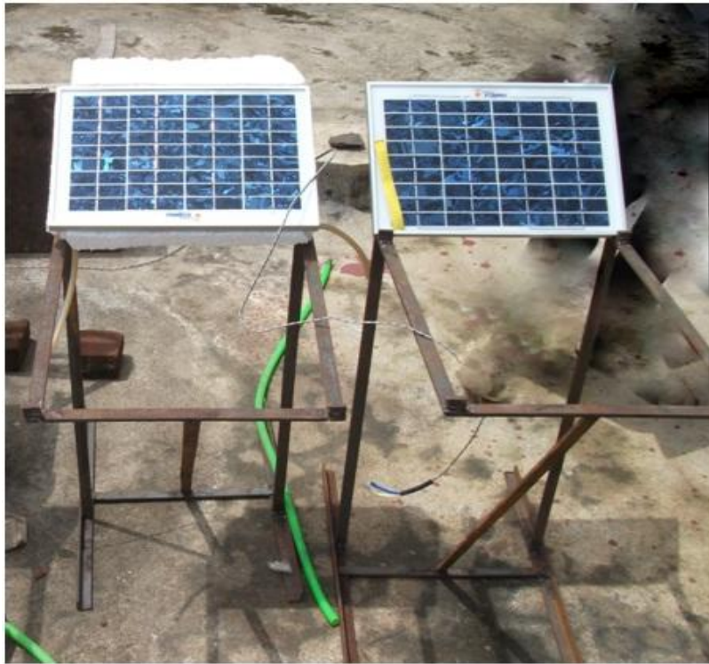
Fig2. Complete experimental set up for water based PV/T system
