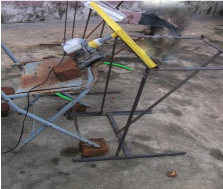
Fig4. Complete experimental set up for air based PV/T system
