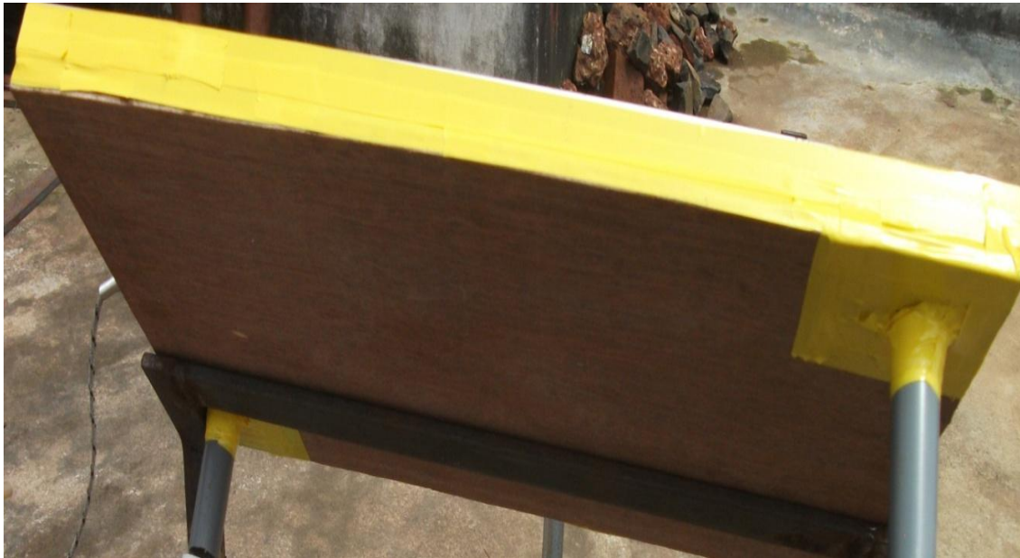
Fig5. Rear side of the solar panel-Air based PV/T system
