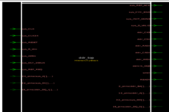
Fig 5. Top level schematic of the Controller
