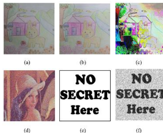
Fig11. Experimental results of Experiment-II: (a) the digitalized share that is captured by Canon 650D digital camera, (b) the digitalized share that is captured by iPhone 4, (c) difference between Fig. 11(a) and Fig. 11(b), (d) recovered image of SE1 (PSNR = 12.12 dB), (e) binary secret image ( SE2 ), (f) recovered image of SE2 (contrast = 60.64%).
