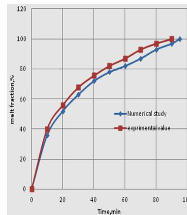
**Fig4.** melts fraction Vs time, spherical geometry
