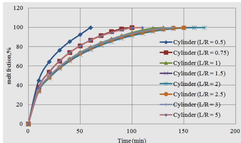
**Fig8.** Comparison of melt fraction for various aspect ratios
