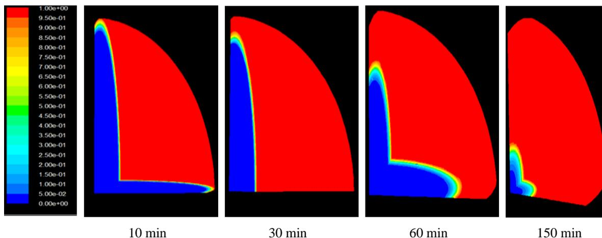
Fig5. Distribution of solid and liquid phases at various times
