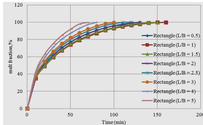
**Fig11.** Comparison of melt fraction in various aspect ratios
