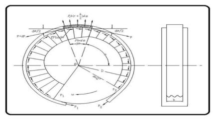
Figure2. Stress analysis of the flexible body
