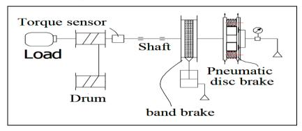
Figure 1. Proposed Setup for analysis of Band Brake
