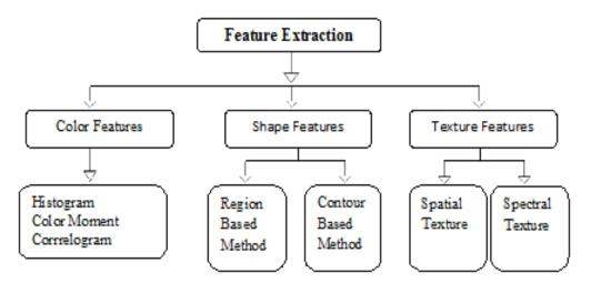
Fig1. Block Diagram of Feature Extraction
