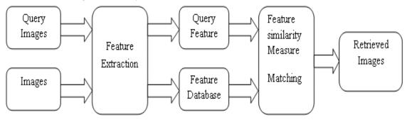
Fig2. Diagram of the Image Retrieval System
