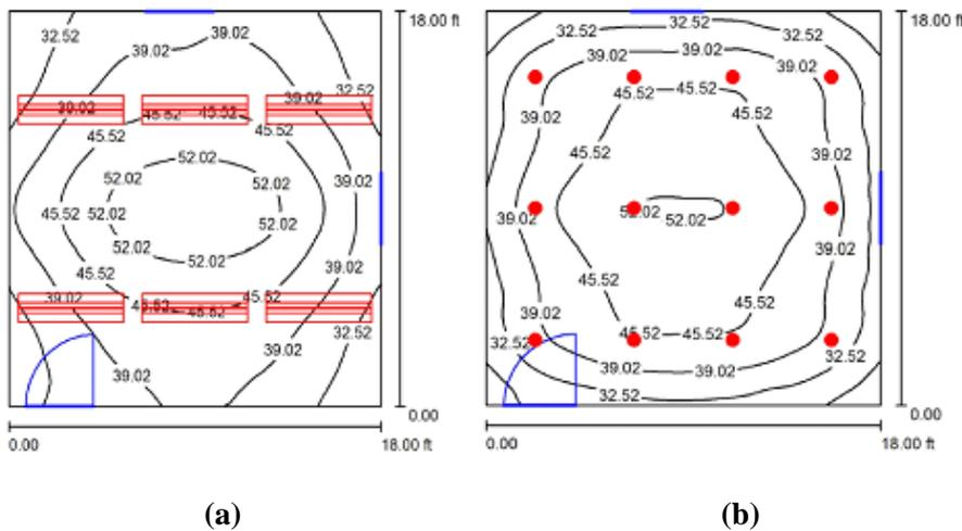
Field arrangement of fluorescent lamps (a) and LED lamps (b)
