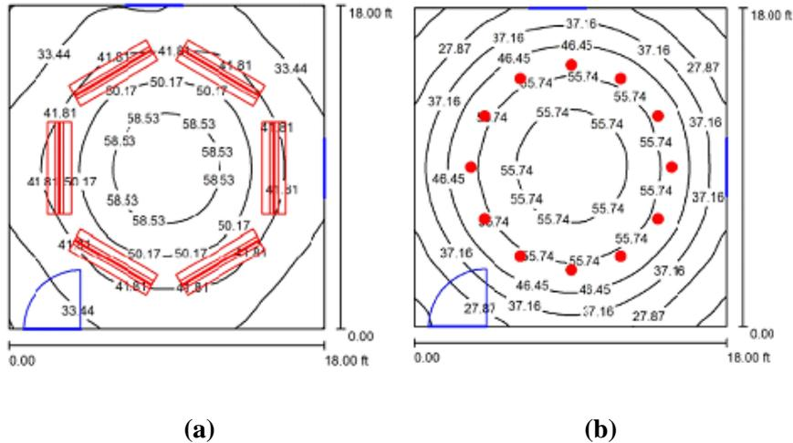
Circle arrangement of fluorescent lamps (a) and LED lamps (b)
