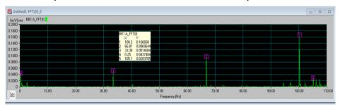
Spectrum at Plummer block no.1 unbalanced 2000 rpm Axial
