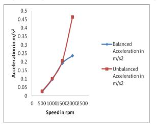
Figure5. Graph for comparison of balanced & unbalanced horizontal position
