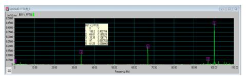
Spectrum at Plummer block no.1 unbalanced 2000 rpm Vertical
