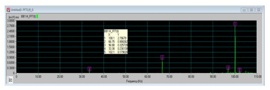
Spectrum at Plummer block no.1 balanced 2000 rpm Horizontal
