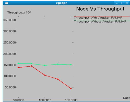
Fig10. Number of nodes Vs Throughput
