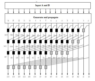
Fig5. Simple 16- bit Kogge stone adder
