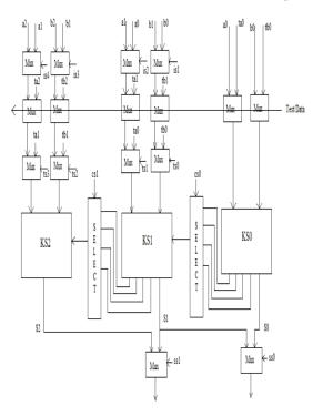
Fig7. Single fault tolerant kogge stone adder
