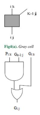
Fig4(b). Logic definition of Gray cell
