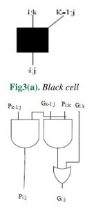
Fig3(b). Logic definition of Black cell
