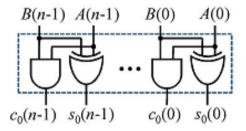
Gate-level optimized design of (CG0) for input-carry=0.
