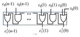
Gate-level design of the CS unit
