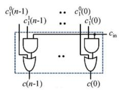
Gate-level design of the final-sum generation (FSG) unit
