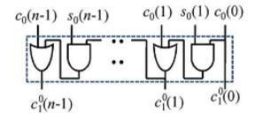
Gate-level optimized design of (CG1) for input-carry=1
