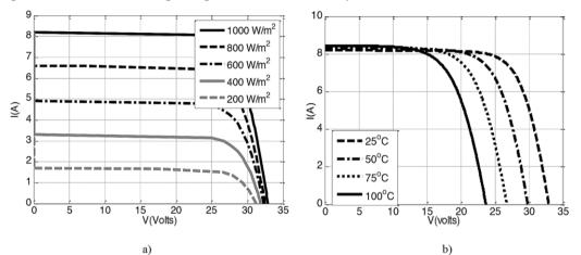
**Fig.I-V.** Characteristics of Kyocera KC200GT of PV module (a) varying irradiance; (b) varying cell temperature.
