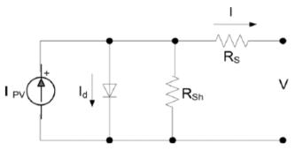
Fig1. One diode equivalent circuit of Solar PV.
