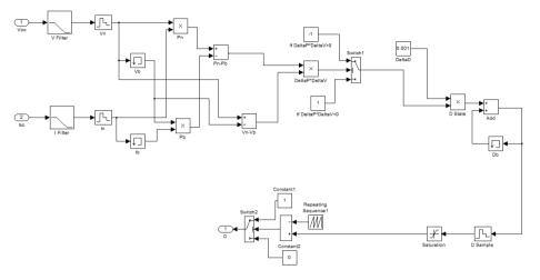
Fig. Simulink Diagram of P & O Method
