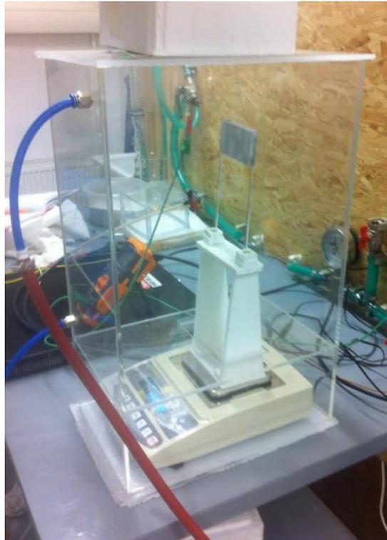
**Figure2.** The whole measuring setup: digital balance, Styrofoam support and the asymmetrical capacitor inside the measuring air-tight chamber.
