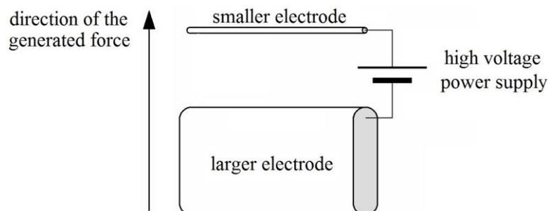
**Figure1.** Principle of the force generated on the asymmetrical capacitor.
