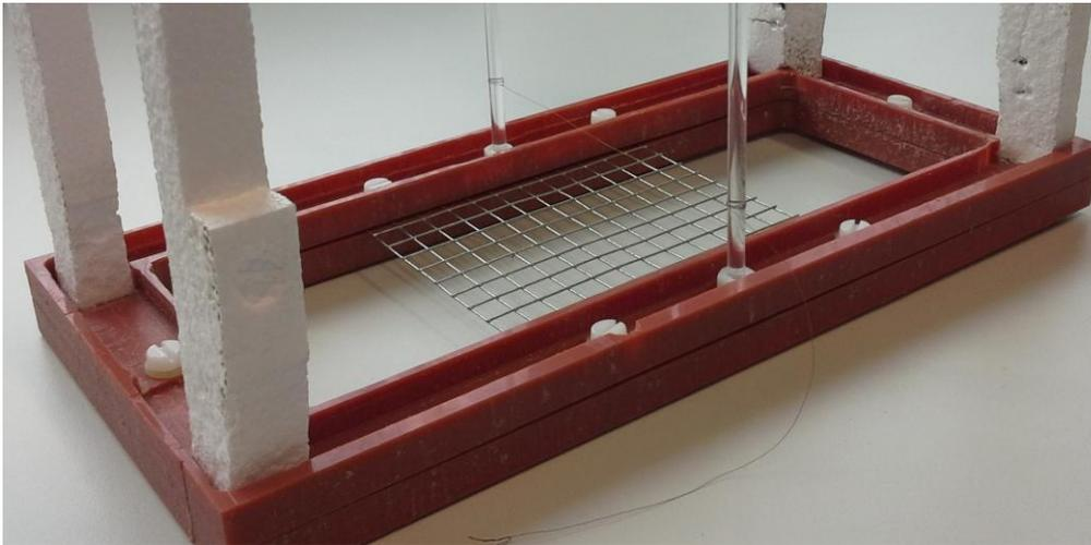
**Figure9.** Picture of the new device, where smaller electrode is still a thin wire, but the larger electrode is no longer solid and is formed by a wire mesh.
