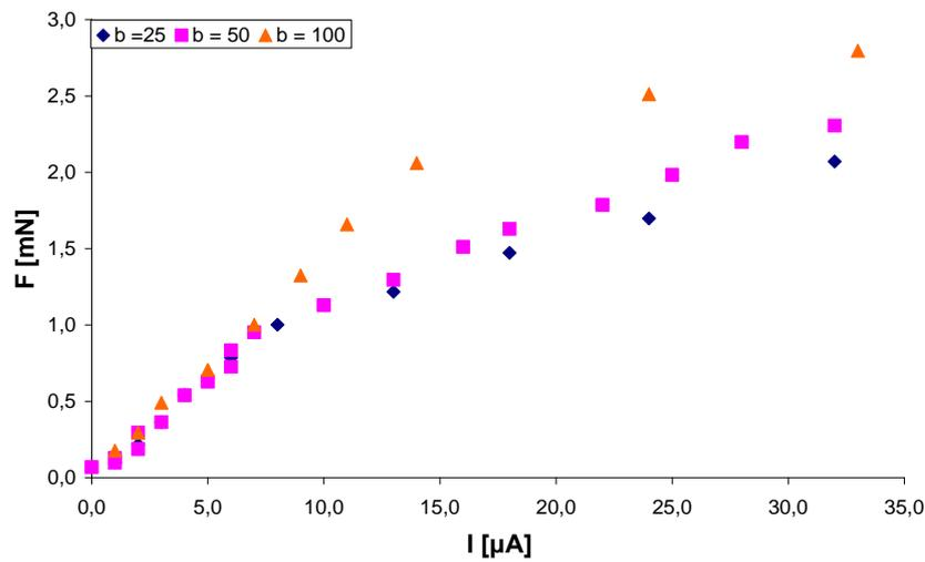
Figure5. Graph representing relation between generated force  $F$  and electrical current  $I$  flowing through the capacitor for capacitors of several values of length  $b$ .
