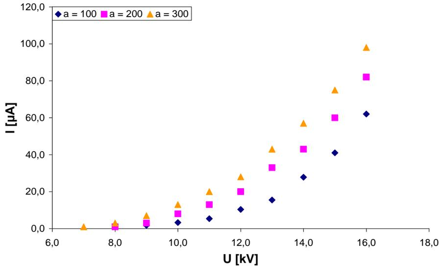
Figure3. Graph representing relation between the electrical current  $I$  flowing through the capacitor and applied voltage  $U$  for capacitors of several values of length  $a$ .
