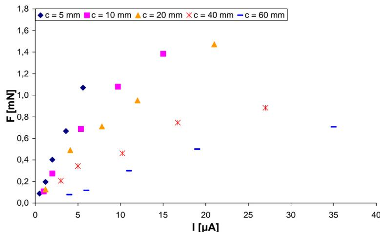
Figure6. Graph representing relation between generated force  $F$  and electrical current  $I$  flowing through the capacitor for capacitors of several values of thickness  $c$ .
