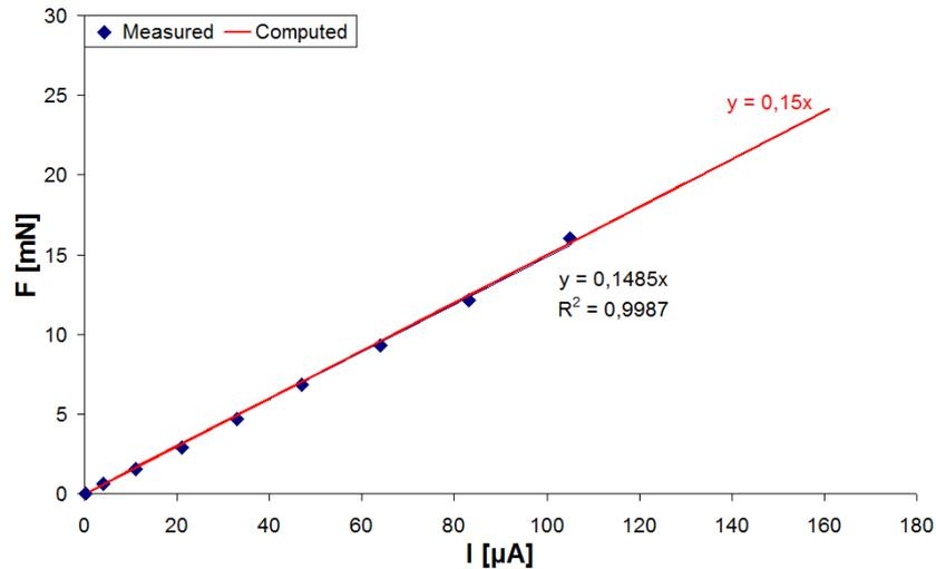
**Figure11.** Graph representing relation between generated force  $F$  and electrical current  $I$  flowing through the capacitor for a capacitor with a wire mesh electrode compared to values obtained using formula (1).
