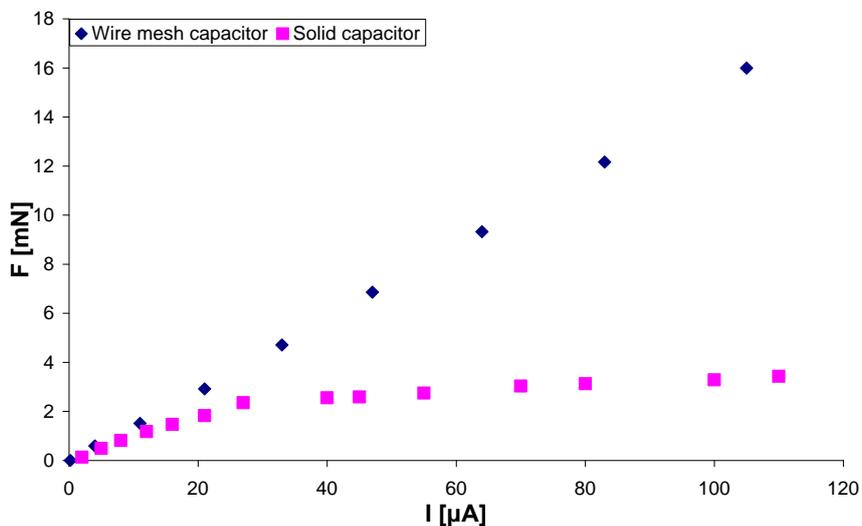
**Figure10.** Graph representing relation between generated force  $F$  and electrical current  $I$  flowing through the capacitor for a capacitor with a solid larger electrode and a capacitor with wire mesh electrode.
