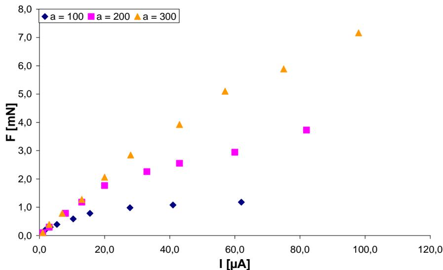
Figure4. Graph representing relation between generated force  $F$  and electrical current  $I$  flowing through the capacitor for capacitors of several values of length  $a$ .
