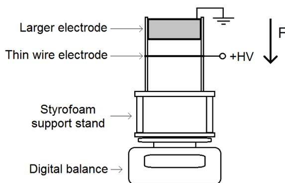
**Figure1.** The whole measuring setup: digital balance, Styrofoam support and the measured asymmetrical capacitor.
