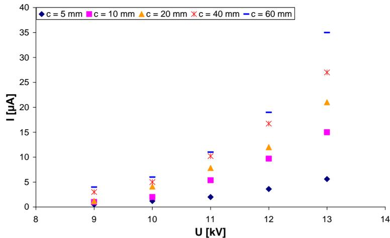
**Figure7.** Graph representing relation between the electrical current  $I$  flowing through the capacitor and applied voltage  $U$  for capacitors of several values of thickness  $c$ .
