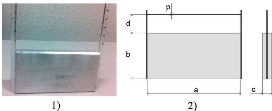
**Figure2.** A picture of 1) the real asymmetrical capacitor with basic dimensions (length  $a = 100$  mm, height  $b = 50$  mm, thickness  $c = 10$  mm), 2) a schematic of the capacitor with highlighted dimensions.
