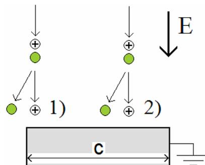
**Figure8.** Schematic representation of two possible behaviour variants of neutral and charged particles in the vicinity of the larger grounded electrode - neutral particle after the collision with the charged particle **1)** misses the electrode, or **2)** hits the electrode and transfers to it the momentum gained from the previous collision.
