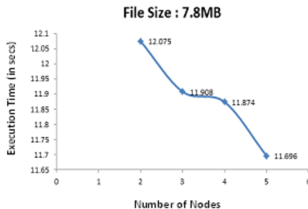
Fig11. Graph for Execution time vs. No. of slave nodes for decompression
