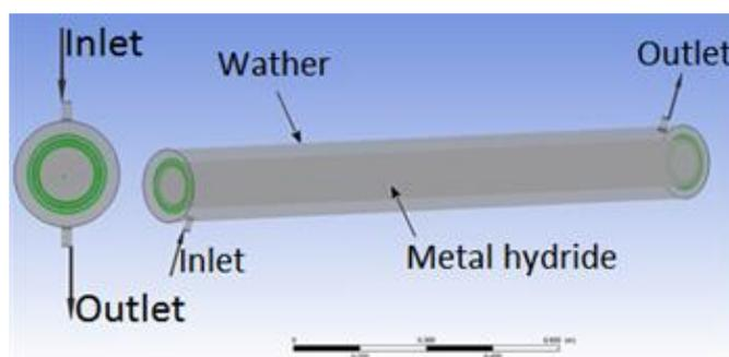
**Figure2.** The geometry of the tray
