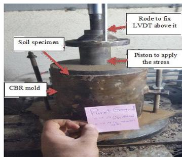
Figure6. Test setup
