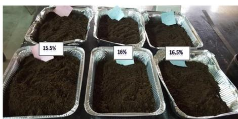
**Figure 3.** Aeration of asphalt stabilized mixture
