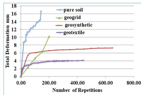
Figure9. Total deformation under wheel tracking test
