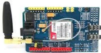
Every carrier or GSM equipment manufacturer must agree upon the Memorandum of Understanding (MoU) before developing the equipment or deploying a GSM based communication system. In this project the GSM module SIM900 is used. This module has an antenna attached to it and requires a 12V adapter to work. The SIM900 delivers GSM/GPRS 850/900/1800/1900MHz for voice, data, SMS and Fax in a small factor form with low power consumption. We are using a 2G SIM for the purpose of communication.
