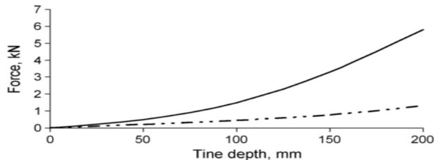
**Figure 7:** Effect of tine depth on the horizontal (solid) and vertical (broken) forces acting on a  $90^\circ$  rake angle tine, *Source:*[8].
