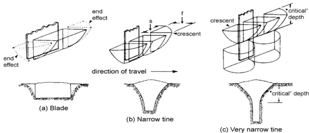
**Figure1:** Effect of implement depth/width ratio on pattern of soil failure; *Source:*[59].
