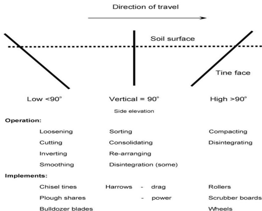
**Figure10:** Optimal tine rake angles for a range of soil operations and basic implements, **Source:**[8]
