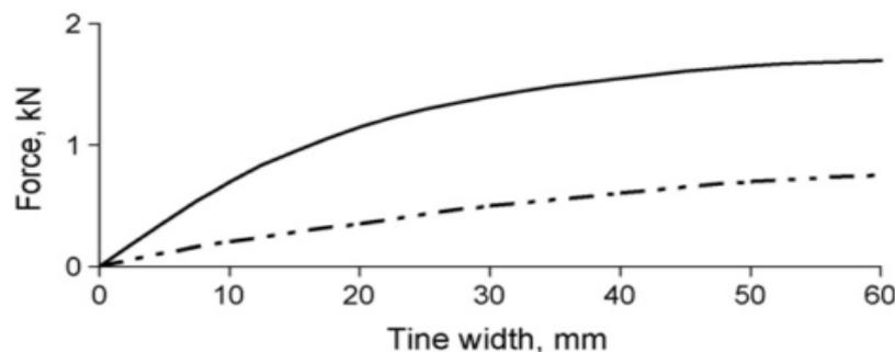
**Figure 8:** Effect of tine width on the horizontal (solid) and vertical (broken) forces acting on a  $90^\circ$  rake angle tine, *Source:*[8].
