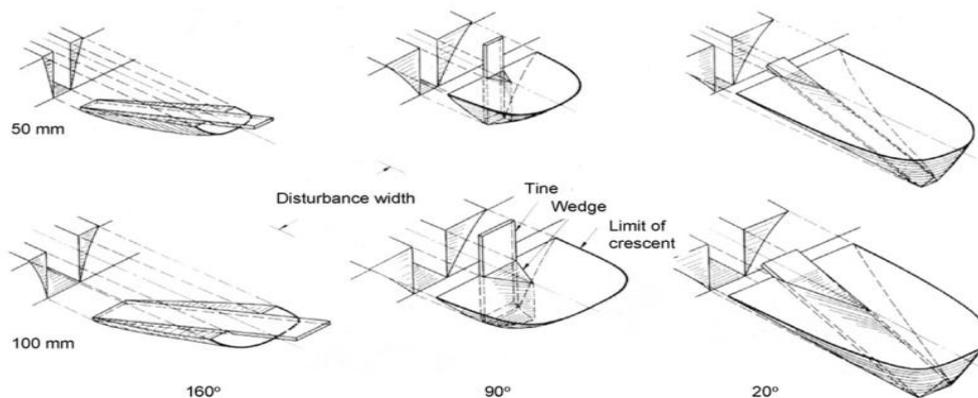
**Figure2:** Effect of rake angle on soil disturbance patterns for tines of 50 mm and 100 mm widths operating at a depth of 150 mm, and  $160^{\circ}$ ,  $90^{\circ}$  and  $20^{\circ}$  rake angles respectively; *Source:*[58]
