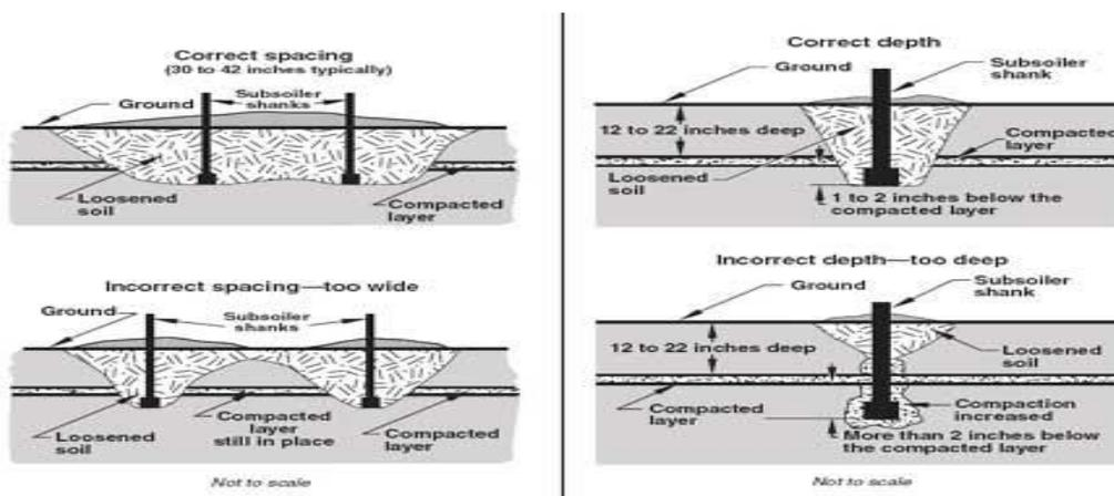
**Figure11:** Correct and incorrect spacing and depth of operation of subsoilers. Source: [43]
