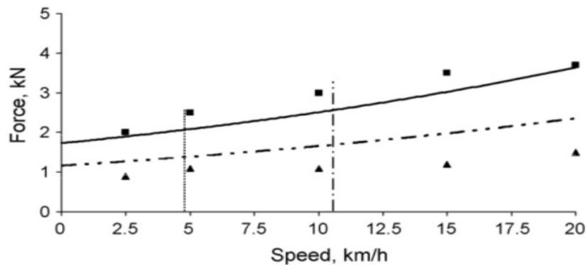
**Figure9:** Effect of tine speed on the measured ( ) and predicted (solid line) horizontal force and the measured ( ) and predicted (broken line) vertical force acting on a 40°-rake angle, 30mm wide, 250mm deep tine in frictional soil; **Source:**[62].
