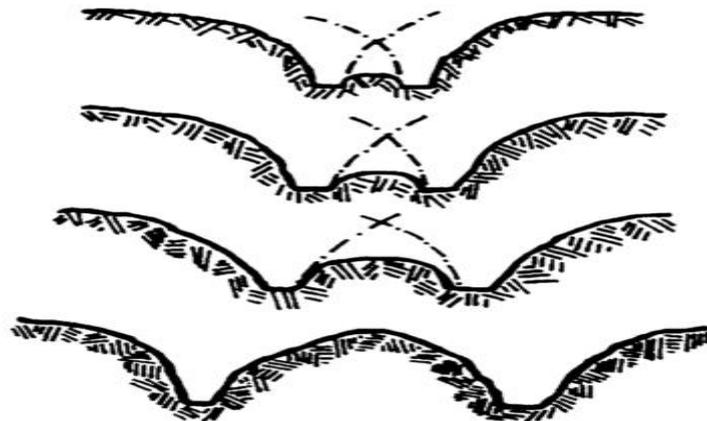
**Figure4:** Profile cross-sections of soil disturbance produced at different tine spacing in a compact sandy loam soil (tine: 25 mm wide, 45° rake angle, 150 mm working depth); **Source:**[7].
