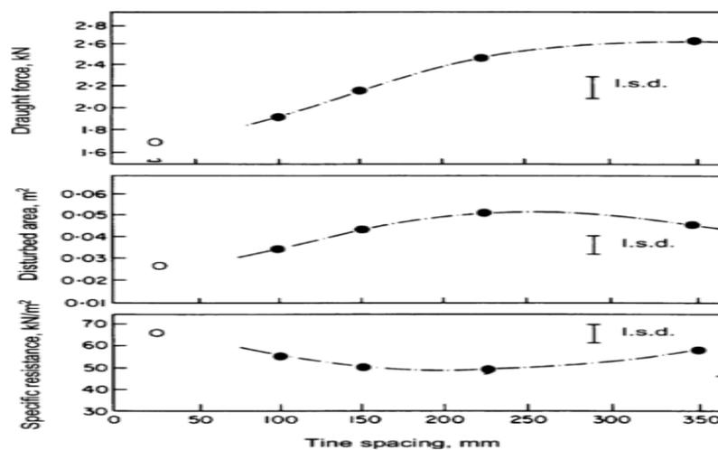
**Figure5:** Relationship between tine spacing and draught force, disturbed area and specific resistance for a pair of 25 mm wide tines operating at 165 mm deep. Open circles represent a single 50 mm wide tine. **Source:**[7].
