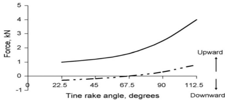
**Figure 6:** Effect of tine rake angle on horizontal (solid) and vertical (broken) forces, *Source:*[8].
