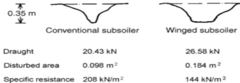
**Figure3:** Effect of adding wings to subsoiler tines on the draught force, soil disturbance pattern and specific resistance in a compact dry clay soil; **Source:**[12].
