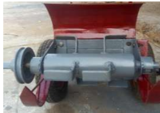
Plate1. The finger type of weeding blade
