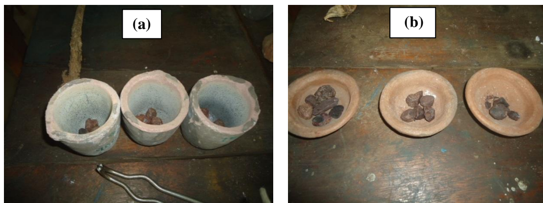
Figure4. Reduction furnace crucibles containing iron ore samples of different sizes (a) Cup-Shaped (b) Hollow-shaped Crucibles
