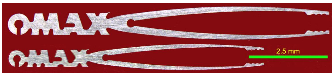
Figure 13. Tweezers machined with 5/10 and 3/8 nozzles
