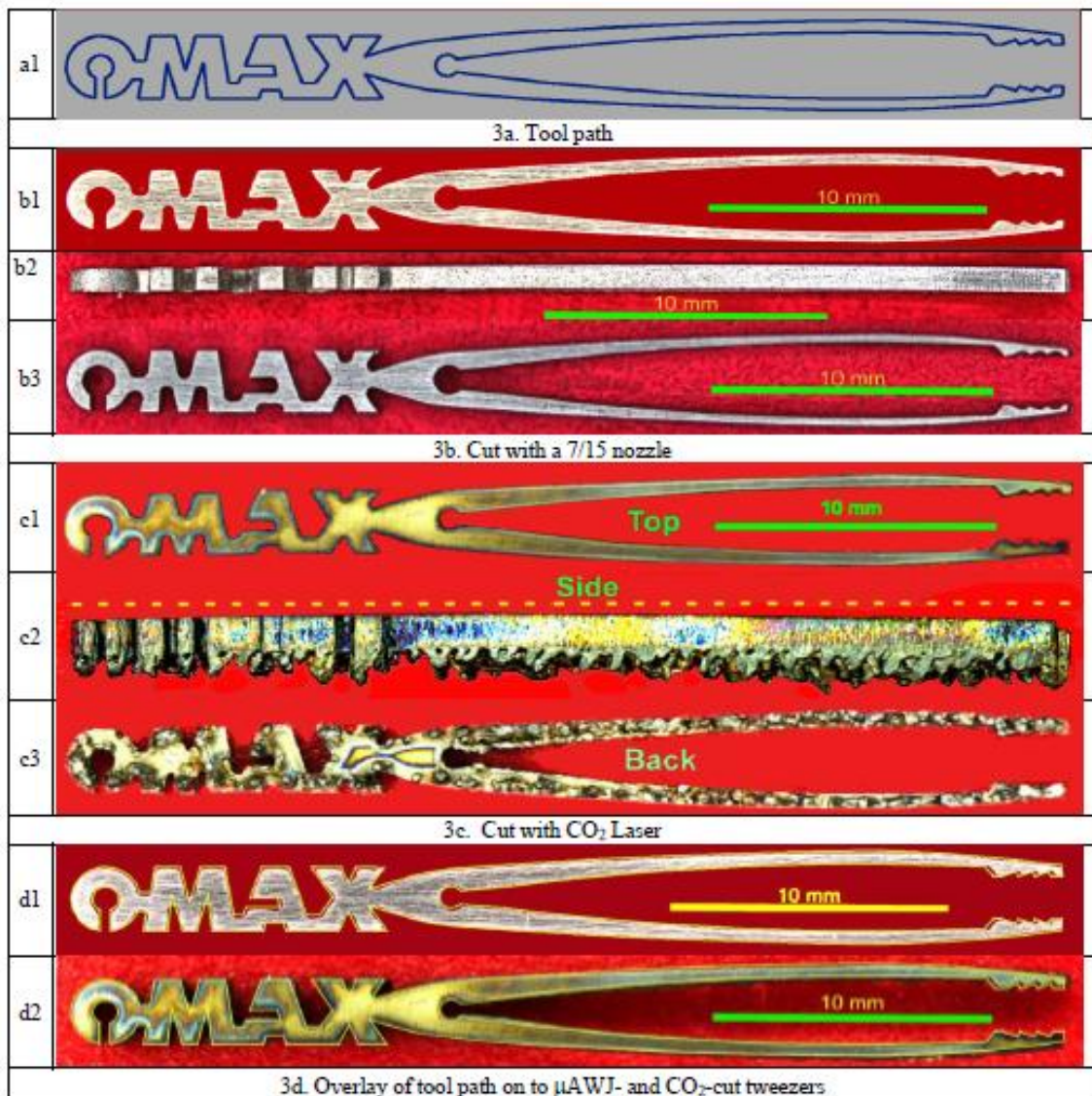
Figure 3. Miniature tweezers cut with \mu AWJ on MicroMAX and CO_2 laser
