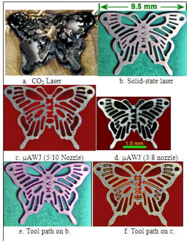
Figure 2. Miniature butterflies cut with lasers and waterjet [3]
