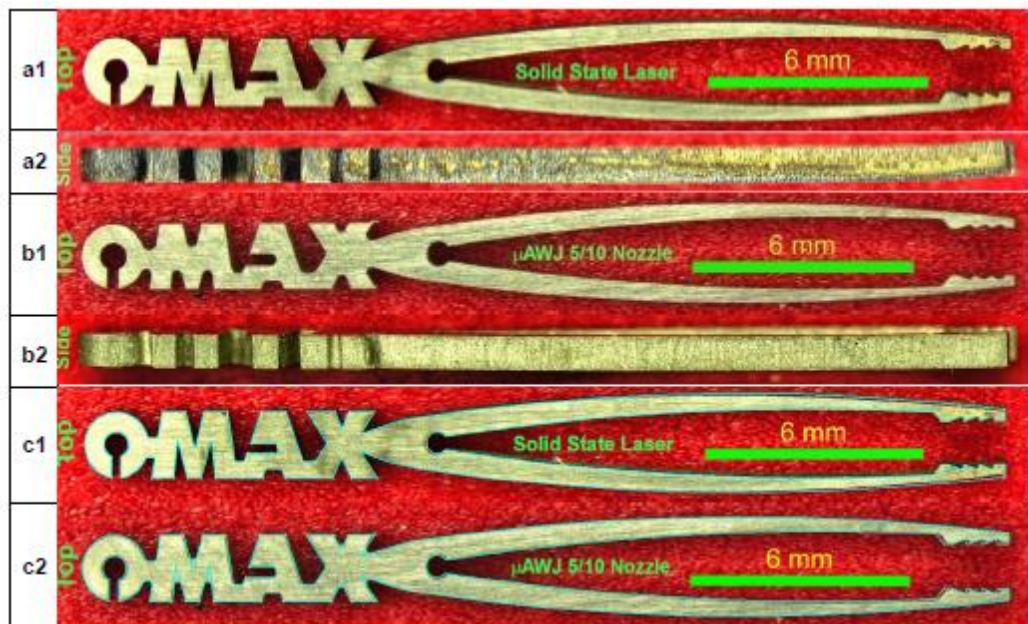
Figure4. Micrographs of miniature Ti tweezers cut with solid-state laser and \mu AWJ with a 5/10 nozzle
