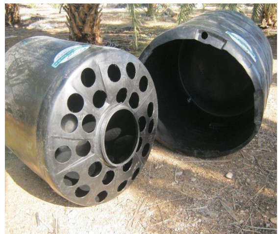
Fig2. A Picture of the External (Right) and Internal (Left) PVC Tanks
