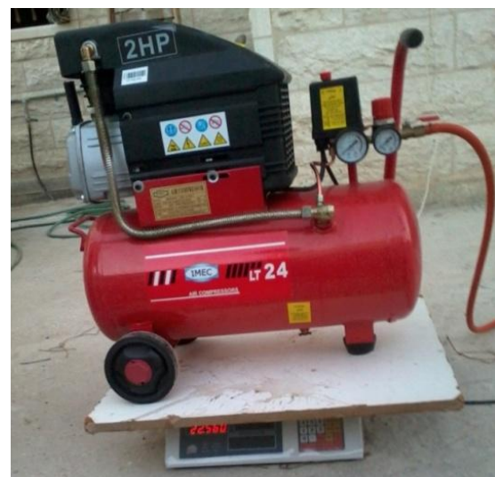
Fig3. The Air Compressor with the Electronic Balance Setting
