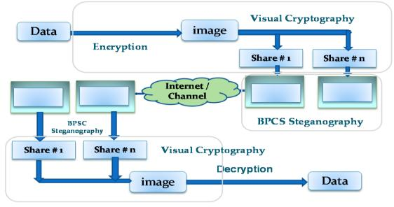
Fig1.3. Architecture of VC and BPCS
