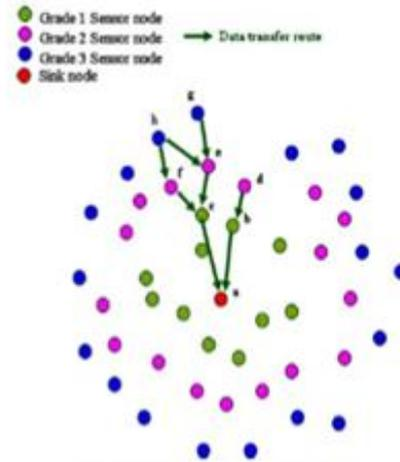
**Fig2.** Data Transfer Route of Sensor Nodes
