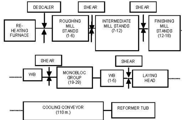
Fig2. Layout of wire and rod mill
