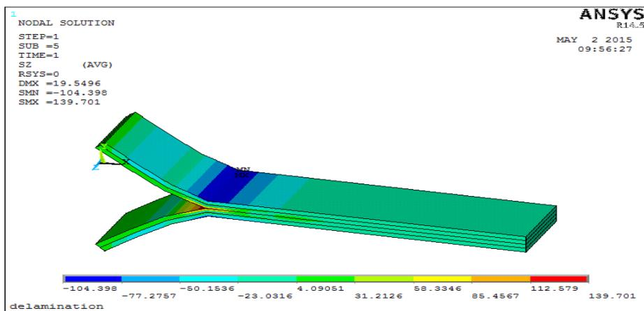
Figure4.3. Z-component of stress with displacement 18mm
