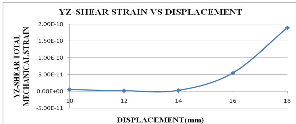
Figure4.15. Variation of YZ-shear total mechanical strain to Displacement
