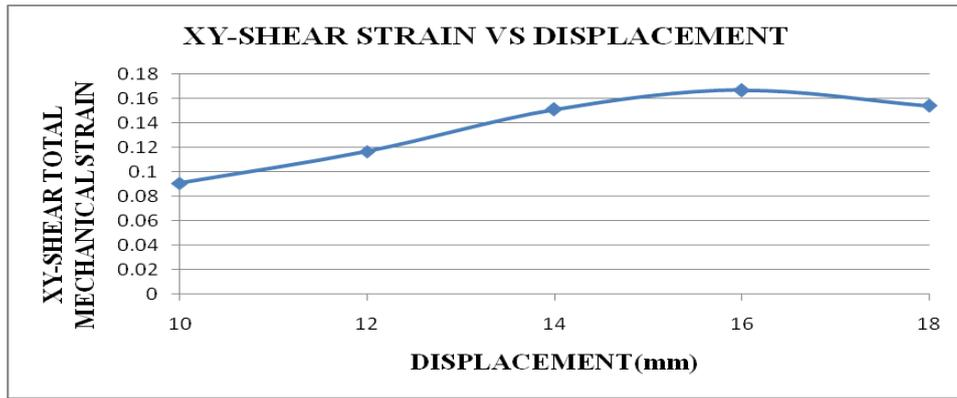
Figure4.14. Variation of XY-shear total mechanical strain to Displacement
