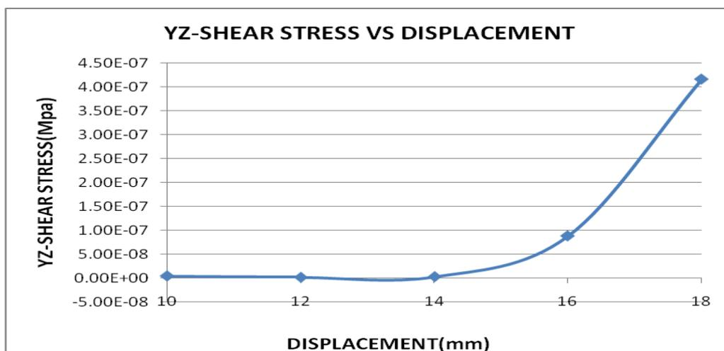
Figure4.9. Variation of YZ-shear stress to Displacement
