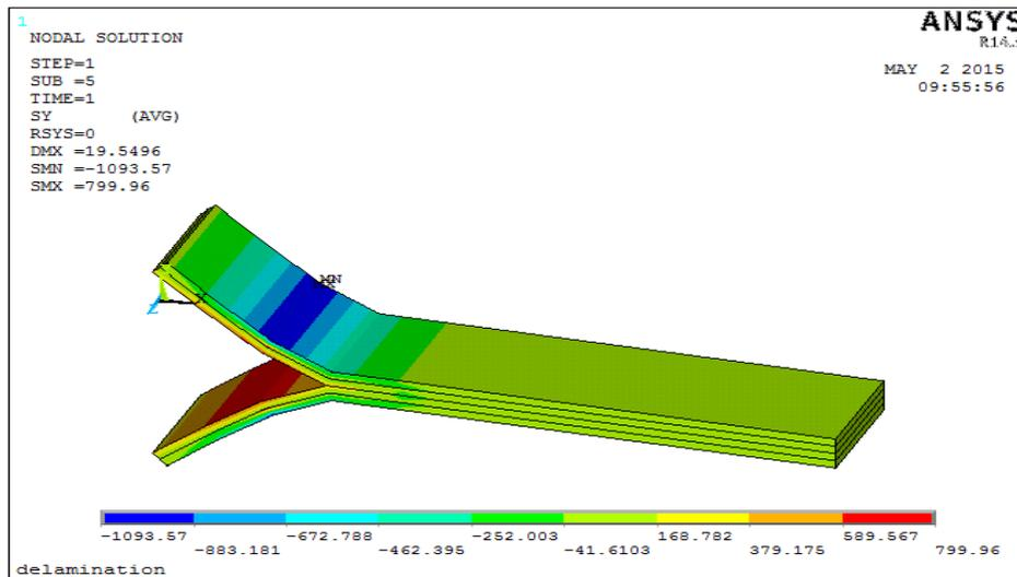
Figure4.2. Y-component of stress with displacement 18mm
