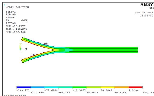
Figure4.1. X-component of stress with displacement 10mm
