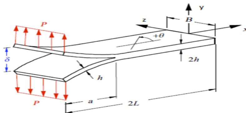
Fig2.1. Specimen for Modeling
