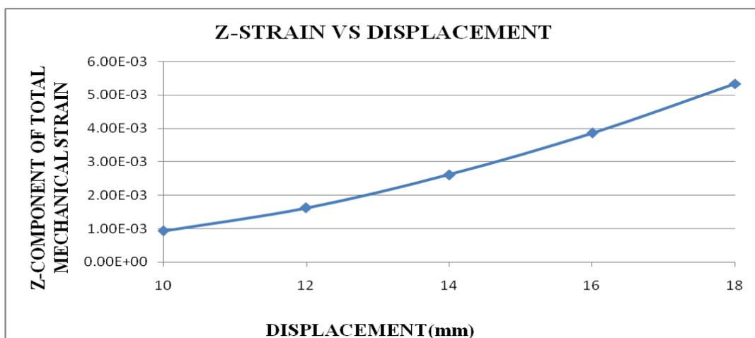
Figure4.13. Variation of Z-component of total mechanical strain to Displacement
